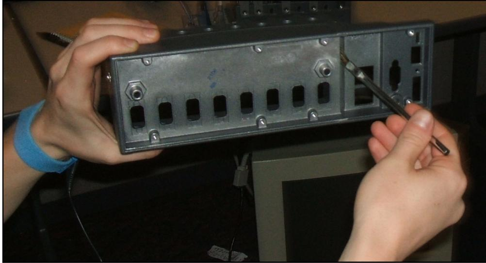
Using a paintbrush to remove foreign objects from the chassis
