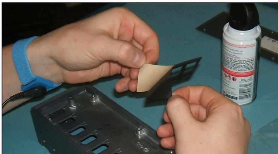
3. Lightly place the gasket in the chassis adhesive side down making sure it is aligned correctly according to the following diagram.
