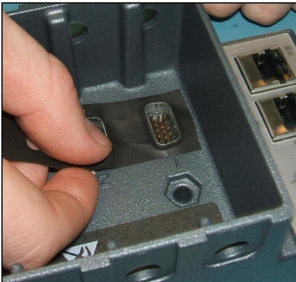
4. Working from the first connector, gently peel away enough of the backing to press the gasket down over each connector, taking care not to stretch the gasket too much.
