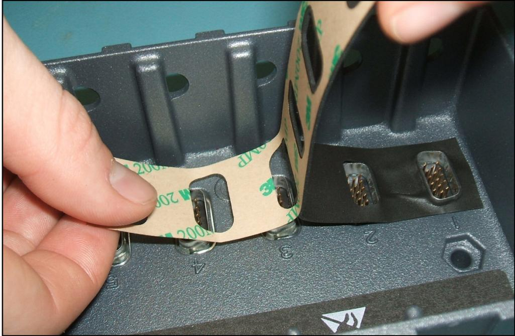
5. When the gasket is in place around all connectors, go back over it and firmly press it into place with a soft, blunt tool.
