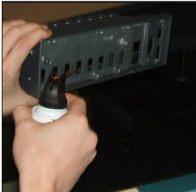
Removing debris from the chassis with compressed air
